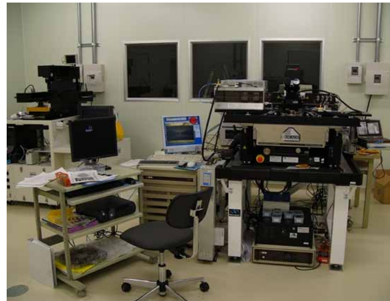
RF measurement system; 8 inch wafer, 40 GHz
