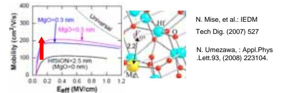
Mobility in Hf-based MOSFET can be improved with **Mg incorporation**.
