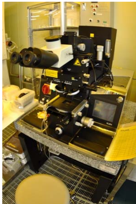
Figure 4.6 The process flow and the photo of photolithography apparatus.
