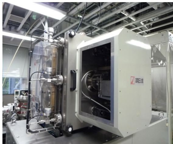
Figure 2.2. Facing Target Sputtering apparatus chamber
