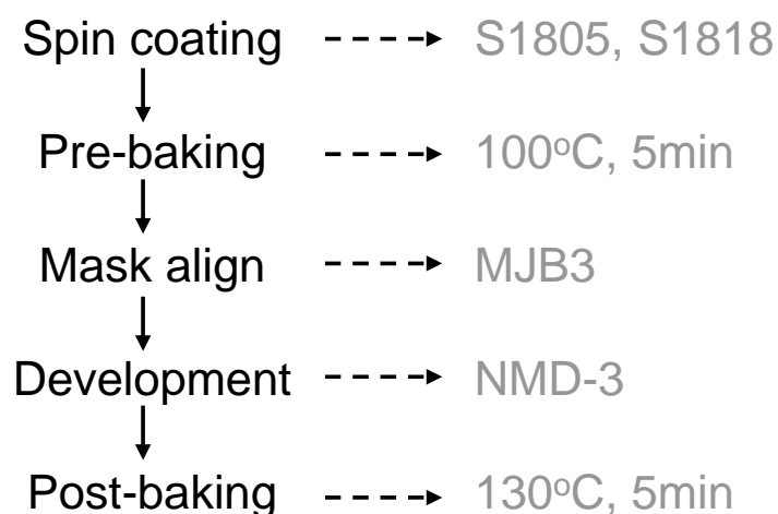
Figure 2-9. Process flow of photolithography.
