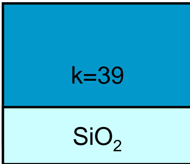
Figure 4.11 laminating structure of k=39 material and SiO 2
