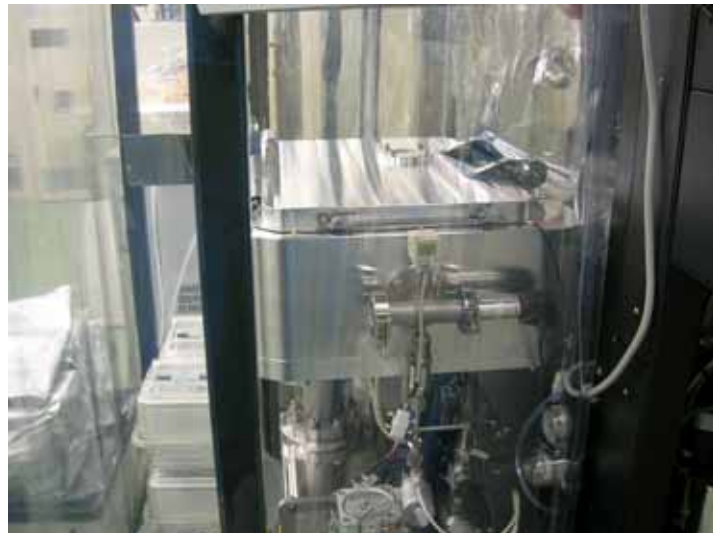
Fig.2.7-ii Photo of Load Lock system
