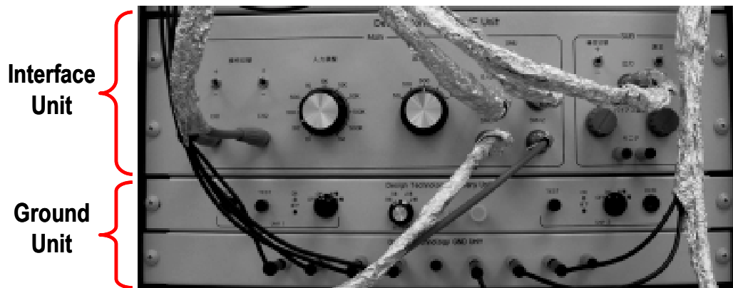
Fig. 3.14 Photograph of 1/f noise interface unit, battery unit and ground unit.
