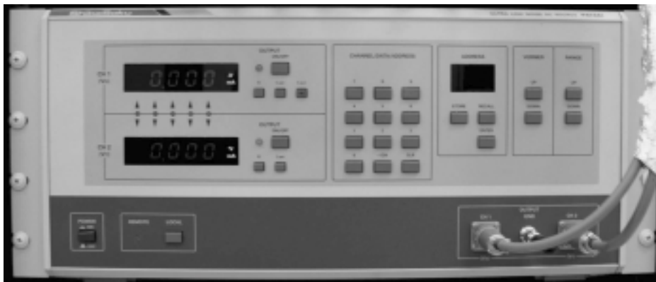
Fig. 3.12 Shibasoku PA14A1 ultra-low noise DC source photograph.
