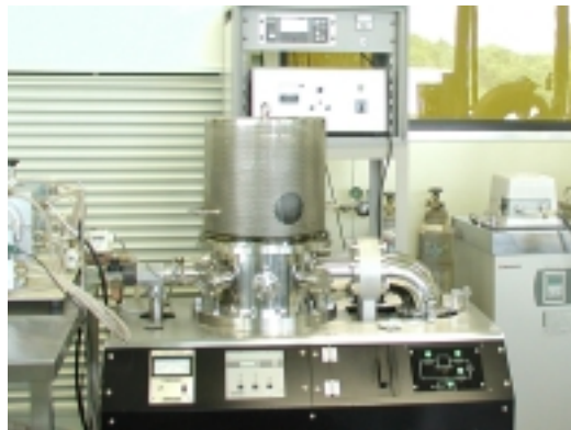
Fig.2.8: High-vacuum bell jar for metal deposition
