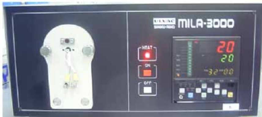
Fig. 2.3. RTA equipment (MILA-3000) used for annealing in O 2 or N 2 .
