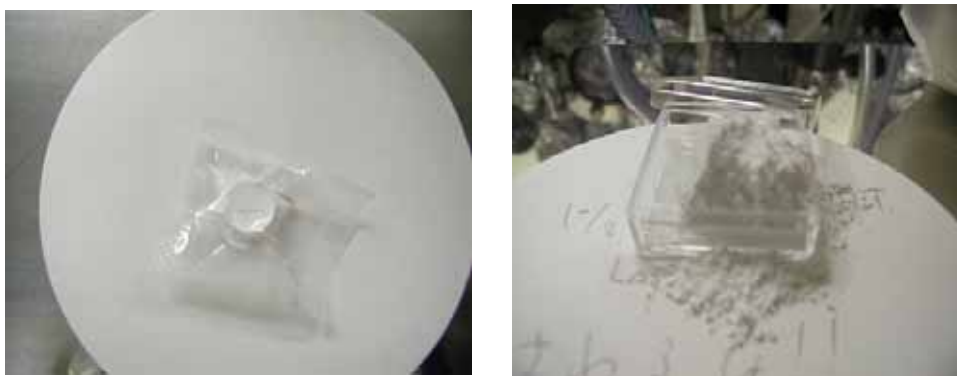
Fig.1.8. La 2 O 3 ceramics (The picture of the left hand is initial, and that of the right hand is after 30 hours in clean room.)
